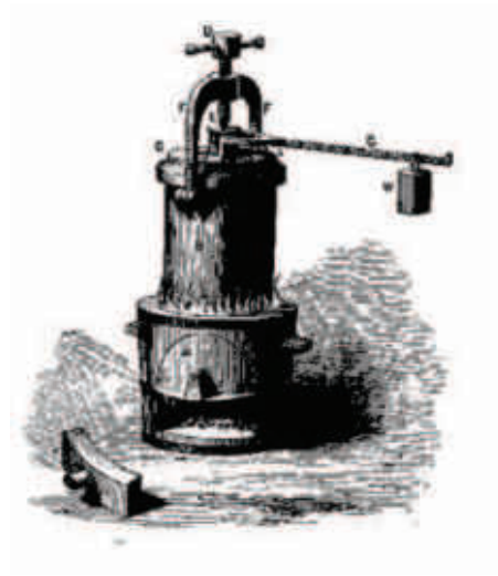
Figure 1.7: French-born inventor Denis Papin (1647-1712) and his steam digester; images from https://en.wikipedia.org/wiki/Denis_Papin .
